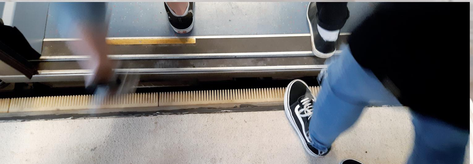
**WILLBRANDT GAP fillers** are the solution for barrier-free entry and exit at platform edges. *GAP fillers* make an important contribution to barrier-free development in local public transport.
